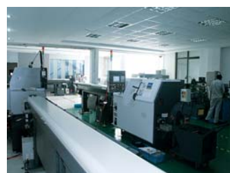
日本进口双主轴车铣复合自动加工中心 Automatic double-spindle turning & milling & boring machining center imported from Japan
