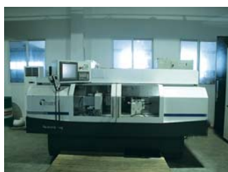
瑞士进口数控精密万能磨床 CNC precision universal grinding machine imported from Switzerland
